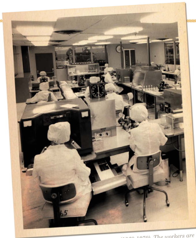
Workers in a lab at Texas Instruments (1960-1970). The workers are wearing white lab coats and white hair coverings. This brightly lighted room in TI's semi-conductor building actually is a photographic “dark room” with yellow illumination. Here, microminiature integrated circuits receive some of their first process steps.
