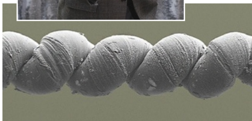
Top: Dr. Ray Baughman. Above: Artificial muscles made from carbon nanotube yarns are infiltrated with paraffin wax and twisted until coils form along their length. The diameter of this coiled yarn is about twice the width of a human hair.
